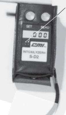
Unique indicator lights show the operator when the subject is providing a sufficient breath sample for analysis. The subject blows through the mouthpiece until both the "A" and "B" lights are illuminated. The operator then presses the "READ" button until the alcohol reading is displayed.
