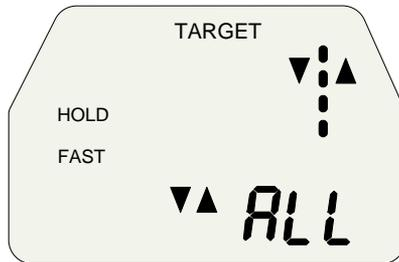
6. Momentarily press the AUD (audio) switch. The TARGET window will display “Aud” and a number from 0 to 5 indicating the audio level will be displayed in the lower right. With “Aud” displayed, press the up (↑) or down (↓) switch to set the audio at the desired level. Also, with “Aud” displayed, pressing the MODE switch will toggle the audio between squelch or unsquelch.
